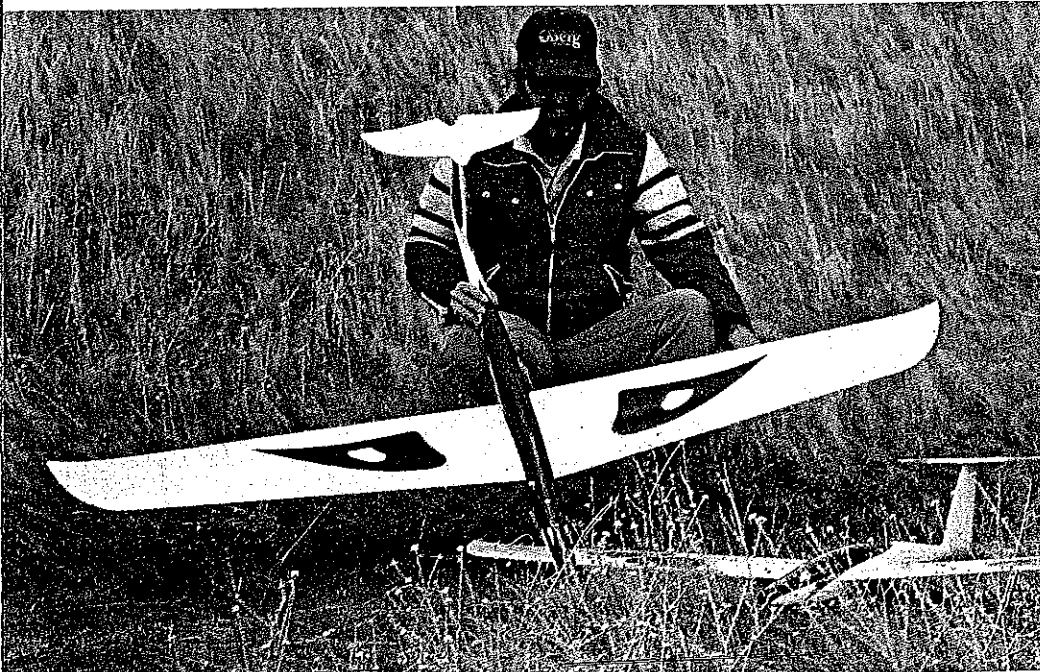
The author's friend Roy Lightel posing with one of two identical Orcas. The shape, distinctive black-and-white color scheme, and pattern design is very reminiscent of its namesake, Orca, the killer whale. An advantage of having no moving control surfaces on the tail feathers is the freedom of design configuration that it allows, as can be seen with the "fish tail" stabilizer.
