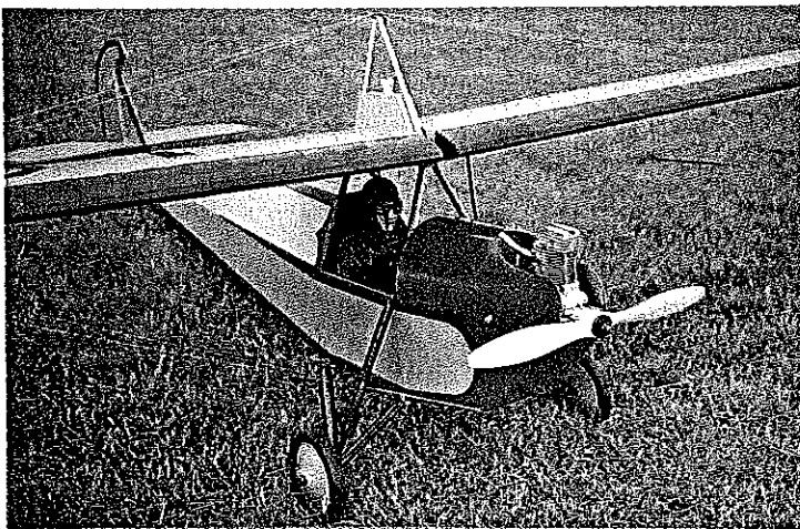
Left: The quarter-scale pilot looks realistic on the ground and in the air. The O.S. Max .40 four-cycle engine is scale in height. Because of the plane's light wing loading, the relatively small engine powers this large model very well. Right: Model is to exact scale and duplicates all parts shown on the plans of the full-size airplane. Fuselage is constructed of birch dowels and spruce. The wing and tail are constructed of balsa.
