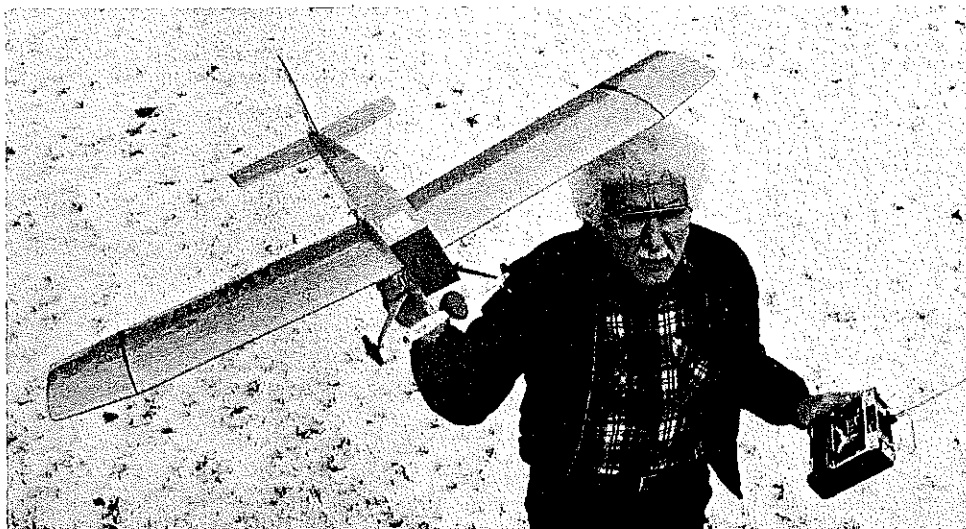
Author/designer Joe Beshar holds the Electrocutor ready for a flight. A bit of fuselage and the landing gear beneath the wing provide for ease of hand launching the almost-low-wing model.
