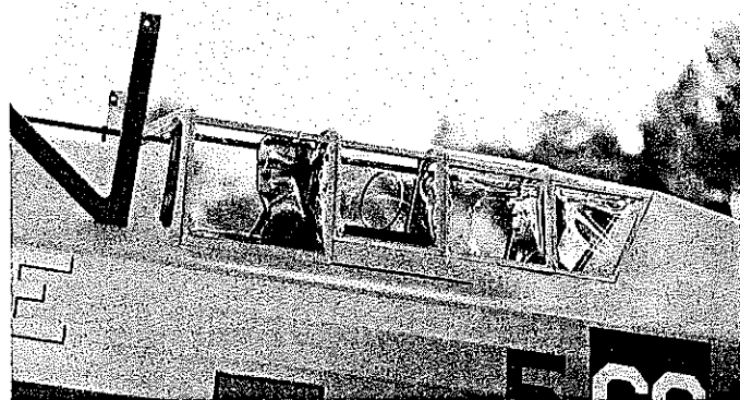
Left: A look at the underside shows how the fillet blocks are contoured into the lower wing and landing gear. Right: Properly sized crew figures help maintain realism. These figures were carved in 1/4-scale, same as the airplane. Loop antenna is for the airplane's radio direction finder.
