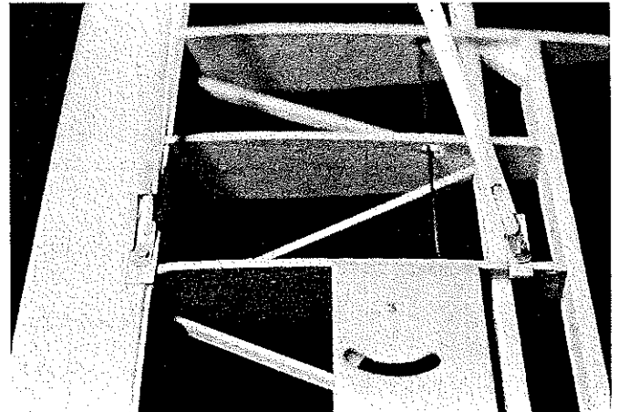
Left: The jury struts are inserted through holes in the small scraps of sheet balsa that are glued flush with the ribs. Right: Carl Goldberg mini snap links fasten the wing struts to brass strips mounted on \frac{1}{16} ply plates that are flush with the ribs. Also note the aileron bellcrank.
