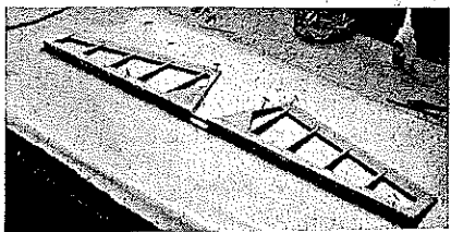
Using the stab as a guide, position the elevator halves. Pin them down and epoxy the brass tie bar in place. Note the airfoil shape.
