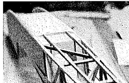
Glue the bottom \frac{1}{4} -in. sheeting and the \frac{1}{4} x \frac{1}{4} stringers into place. Note how the transition from round corners on the sheet to the stringers has been sanded into the sheeting.
