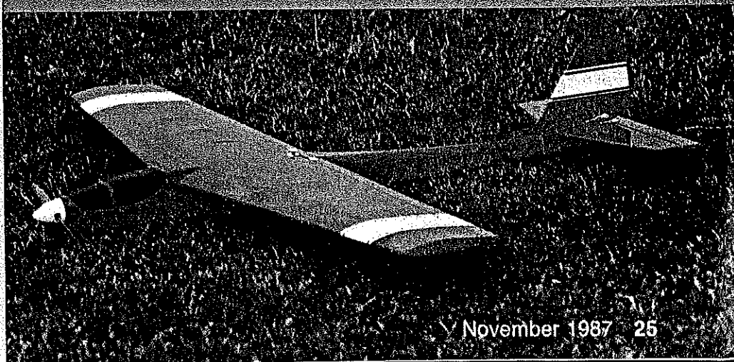
Top: The basically all-red color scheme is simple, light, and shows up well in the air. A little white and black trim on the upper surface helps to tell which side is which during aerobatics. Above: A flyby shows the sleek lines of the Electrostream. The long tail moment provides excellent stability, yet surprisingly allows a crisp snap-roll and spin with immediate recovery. Below: Tom's model has been mistaken for a slope soarer; it might make a good one at that.
