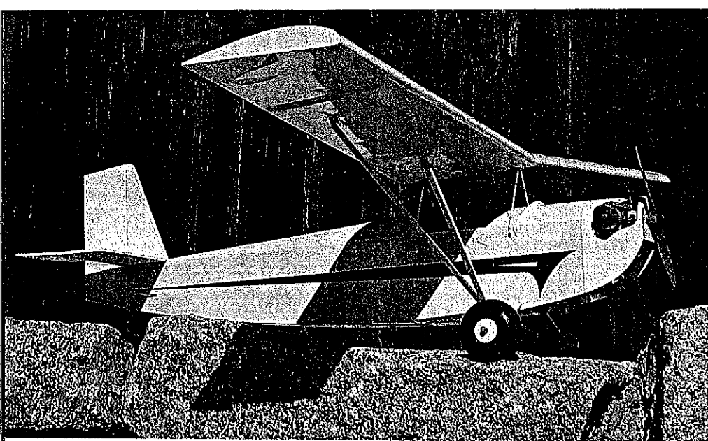
Airfoil is the old standby 15% Clark Y, and the 8-in. chord with 48-in. span means it has an aspect ratio of 6:1. At the prototype's 48-oz. weight, the wing loading is 18 oz./sq. ft. Engine installed is an O.S. .20 two-stroke. By moving the cowl ring forward slightly, a .20 four-stroke engine would be an excellent choice for the power plant. All photographs by the author.
