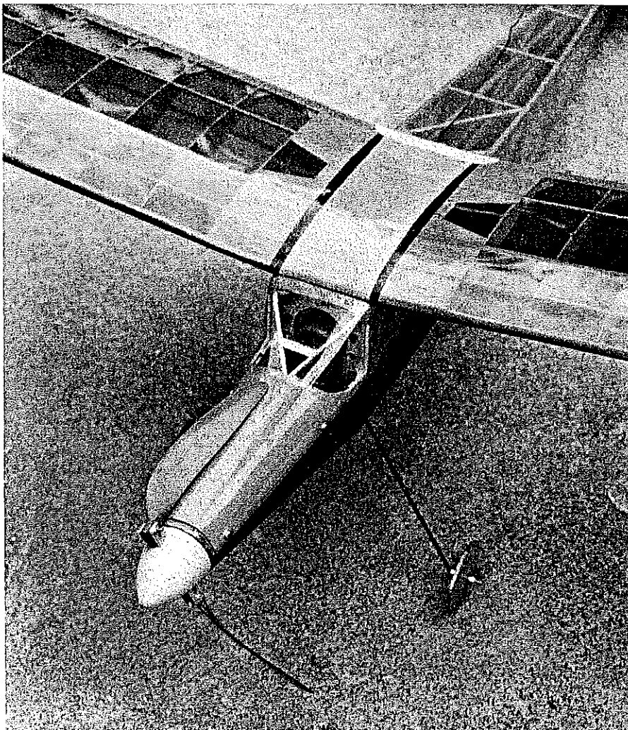
Clean, wouldn't you say? Turbulator spar is at 15% of chord. Top and bottom spars are flat spruce with center webbing—has withstood vertical dives and pullouts. Rear top spar helps to control warps. Folding prop blades shouldn't swing forward of the normal path; if your hub allows a more forward pivot, always launch with the nose slightly up (you'd better!).
