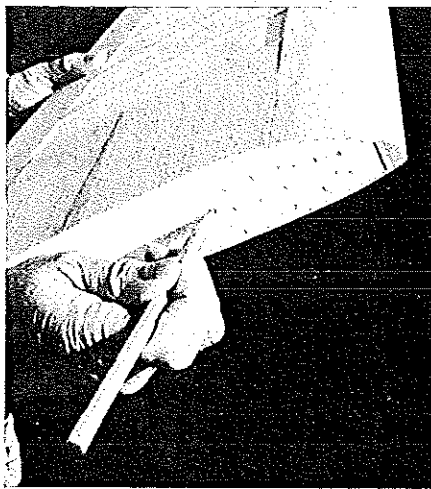
Strengthen wing by punching holes into the roots before joining the halves with epoxy.
