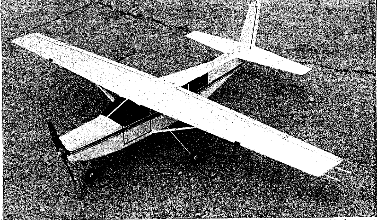
Good moments and generous areas make this an ideal design for Control Line. The tricycle landing gear provides very smooth landings.
