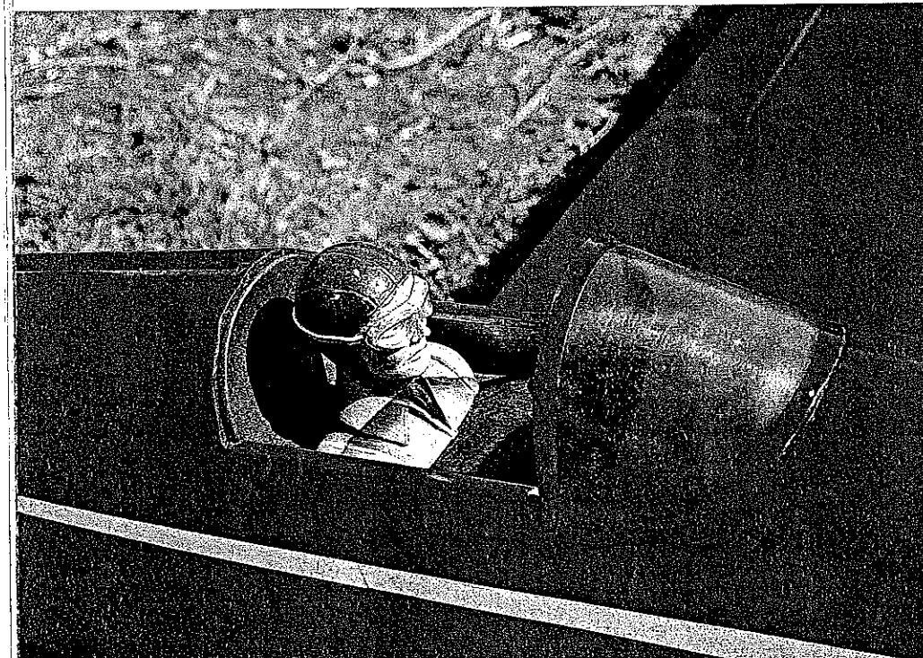
The 2-in. Williams Bros. standard pilot really completes the model, especially in flight. The receiver switch is also in the cockpit, located just ahead of the pilot. Little dots of epoxy were applied to the windshield before the framework was painted for simulation of the rivets.
