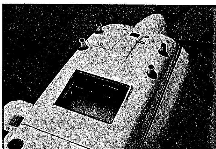
Left: Wheel pants are constructed using foam, glass cloth, and epoxy (more details in the text). The landing gear is fitted after the wing is removed from the jig. Right: Lip on edges of the air exit add to the realism. Exhaust stacks are aluminum tubes sunk into balsa and held with epoxy glue. Black dope around the tubes simulates openings in the cowl. Photos of the model by the author and Leon Folsie.
