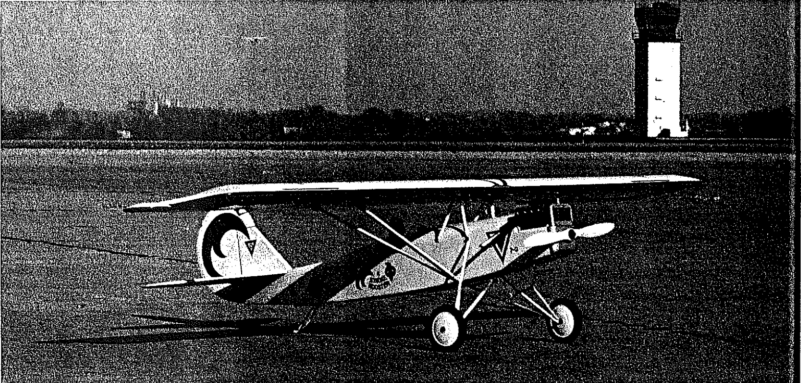
Sitting on the tarmac of the local airport affords us a good view of the struts and landing gear assemblies. Wing construction is a mixture of foam and open framework. Otherwise, the structure is built from balsa and plywood. The four-stroke engine produces a pleasing sound.
