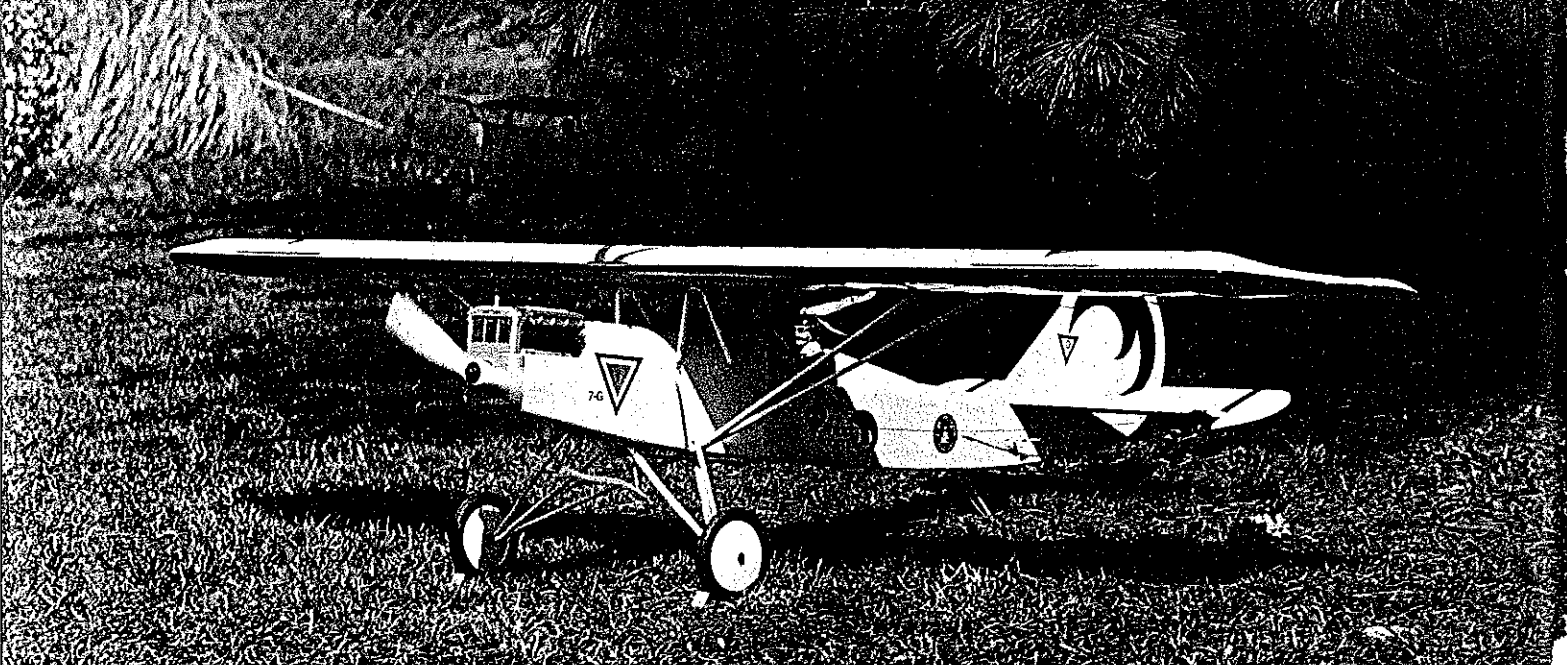
Enya .90 being given a test run in the backyard, the prop just ticking over. Pilot was constructed from open-cell blue foam, clothes made from paper towel material that was later finished with enamel and Hobbypoxy. Featured model evolved from six prototypes before it.
