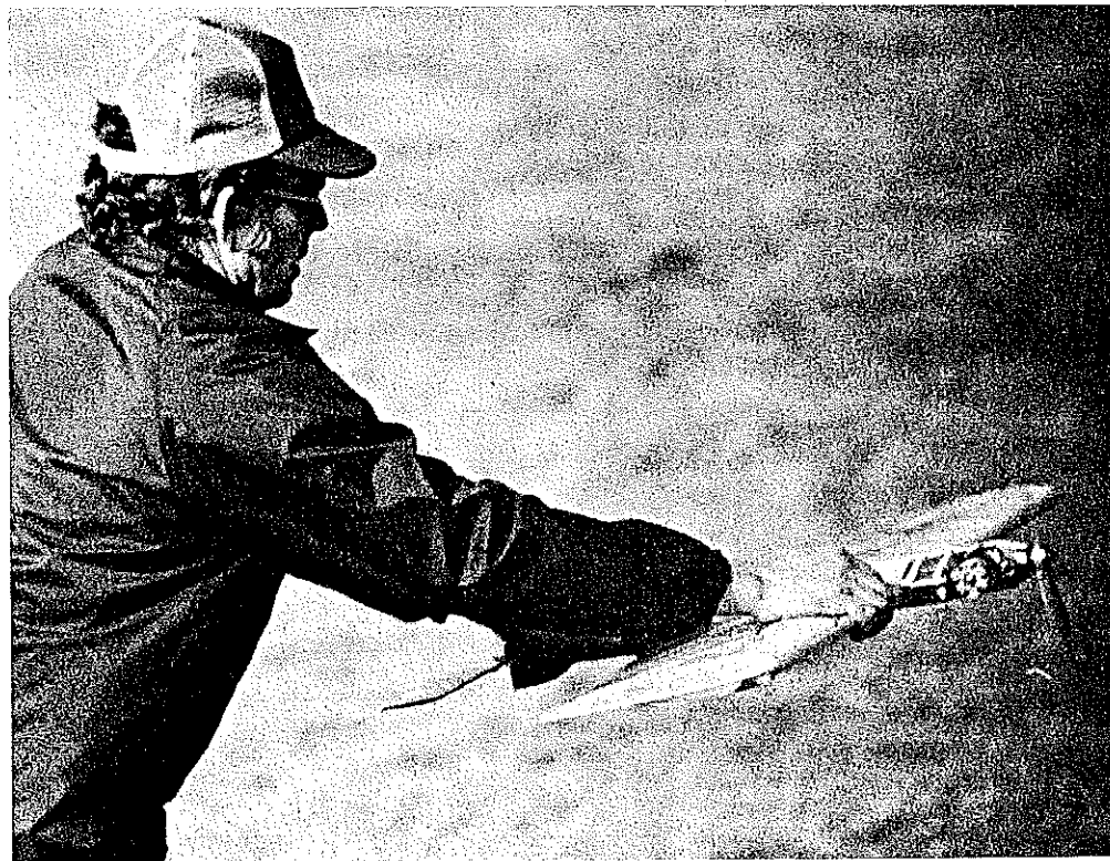
John Hunton launches a Geophysical. Tie-wraps are used to hold the fuel tank securely to the fuselage, providing easy tank removal and replacement. The Geo would be an excellent sport model or Stunt trainer by adding a single-wheel gear and a much more tame engine.
