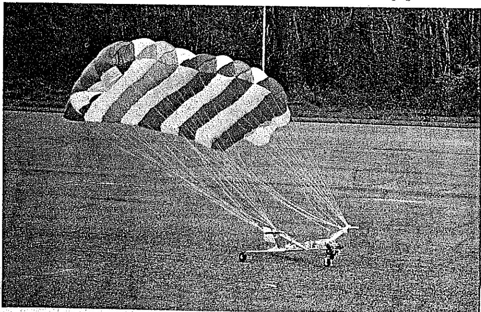
The second ParaCraft was a breadboard designed that seemed too ugly to fly. However, the half-inch plywood fuselage and scrap tail surfaces, with exposed radio gear and tank, were functional for positioning equipment and surviving crashes. Once the best dimensions were discovered, this one was returned to the scrap heap from which it originated.
