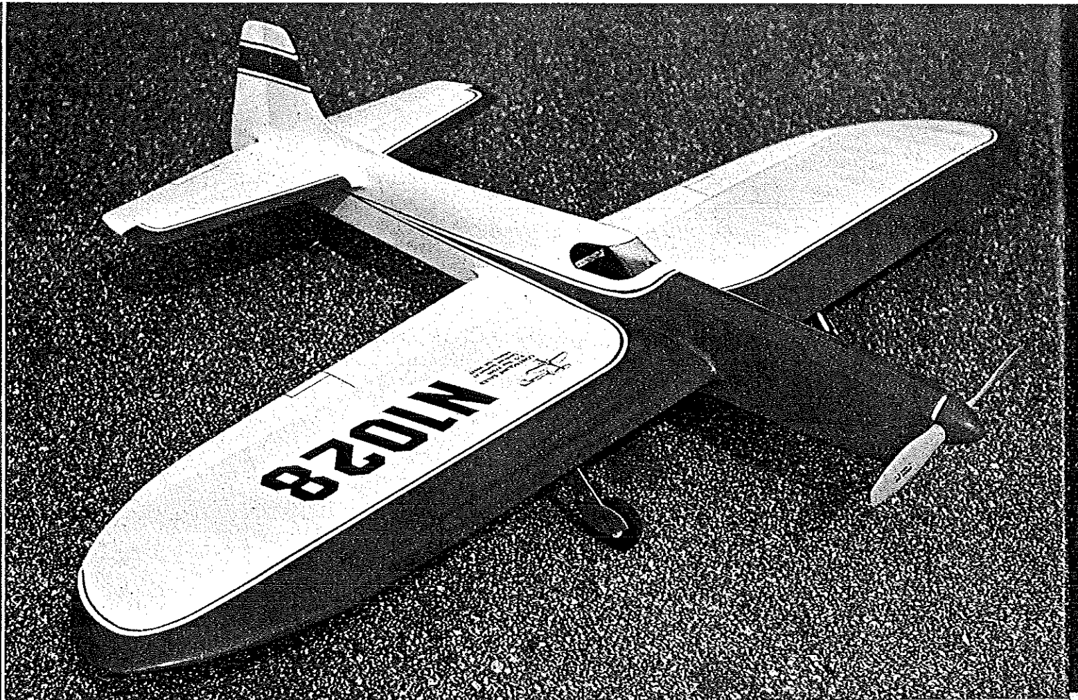
A modern landing gear mounted in the wing provides better takeoffs and landings than the original Smoothie's in-fuselage version. A small piece of paper in the cockpit says, "The pilot is out." AMA numbers are Coverite's stick-on vinyl covered with Sig Lite Coat clear dope.
