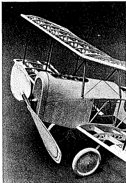
Left: Radiator/nose block unit is made from basswood (carves nicely and resists damage). Top of the dummy Fiat engine is made from either balsa or Styrofoam. Right: The framework design shows concern for choice of wood sizes to achieve optimum strength relative to weight. Points of high stress, such as at the wing roots and landing gear, are given special attention. Author is a master of the Rubber Scale art.
