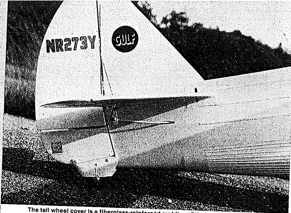
The tail wheel cover is a fiberglass-reinforced molding. Other things to see are the stringers on the fuselage side and bottom, dummy tail light, and location of the tail brace wires.
