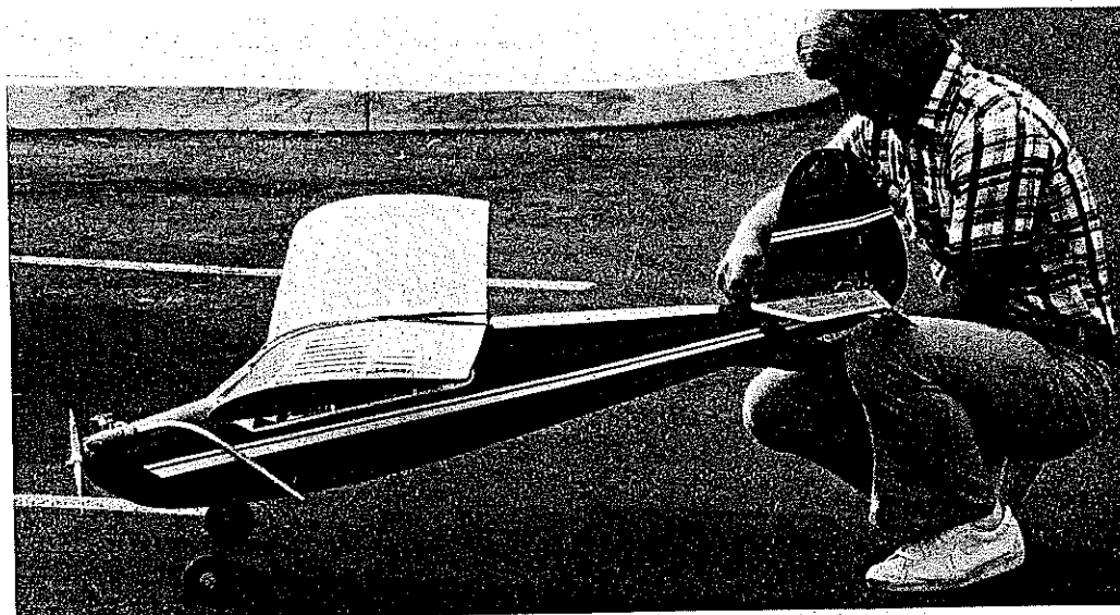
John Laycock hooks up the rubberbands to hold the tail section. This is an early picture when the landing gear of 1/8-in. music wire and Trexler wheels was in use. Being too springy, the author changed to 5/32-in. wire and low-bounce wheels. That did the trick very nicely.
