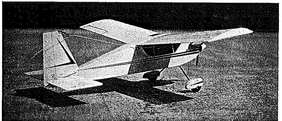
MonoKote trim applied to the fuselage, rudder, and wheel pants is easy to apply, looks great.
