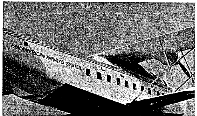
Left: Round 1/8-in. brass tubing soldered into the middle of streamlined brass tubing diagonal struts provides sockets for 1/8-in. dowel vertical struts. All doped silver. Right: Windows are cut from 1/16-in. Plexiglas; corners are sanded round. Bumps above the row of windows simulate air vents. Lettering is cut from black Super MonoKote as per the method described in the text. You may never paint your lettering again.
