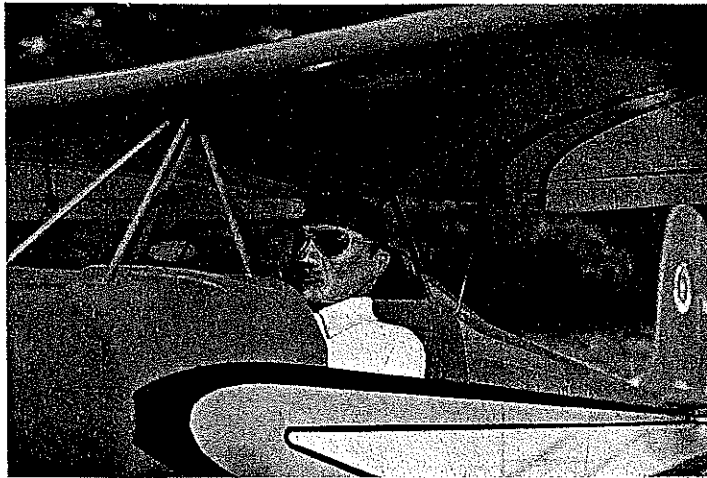
Head and chest of the carved balsa dummy pilot rest on a plywood platform fastened to rails in cockpit. Chin to head top is about 2 in.
