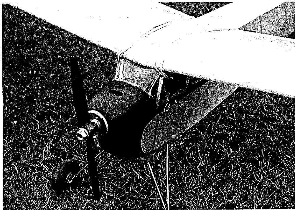
The model is flown on a 7-3 prop, but props from 6-4 to 7-4 work okay. An RC-controlled on-off switch is a virtual necessity to prevent the possibility of motor damage (and for soaring).
