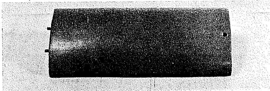
The bottom hatch can either be built-up (for minimum weight) or carved from a solid balsa block.
