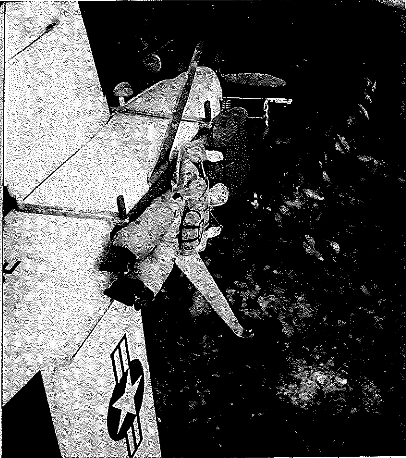
These pictures show two different chute pods used on the author's Snapshot 2 plane—and two locations for the chutist. In any case, the pod should be sanded smooth to prevent fabric snags. With chutist on 72 MHz and the model on 53 MHz, the close proximity of receivers has not caused interference—while some same-band combinations have been troublesome in this regard. In the photo at right with the author's wife, Dawn, can be seen the mirror on the fuselage which allows the camera to look rearward (but the pilot has to be quick on the shutter for close-ups of releases).
