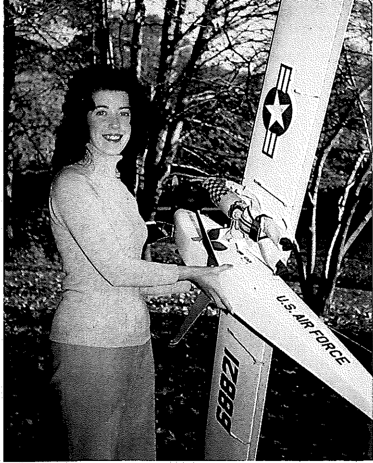
These pictures show two different chute pods used on the author's Snapshot 2 plane—and two locations for the chutist. In any case, the pod should be sanded smooth to prevent fabric snags. With chutist on 72 MHz and the model on 53 MHz, the close proximity of receivers has not caused interference—while some same-band combinations have been troublesome in this regard. In the photo at right with the author's wife, Dawn, can be seen the mirror on the fuselage which allows the camera to look rearward (but the pilot has to be quick on the shutter for close-ups of releases).
