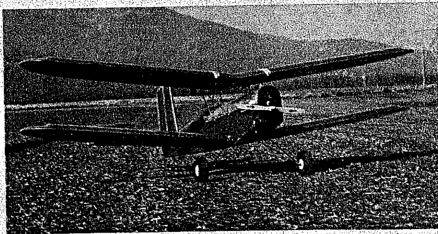
Broad landing gear and large wheels allow operation from grass fields. Brace wires are joined in center by rubberbands wrapped to provide shock absorption during rough-field operations. Big wing area makes for soft landings.
