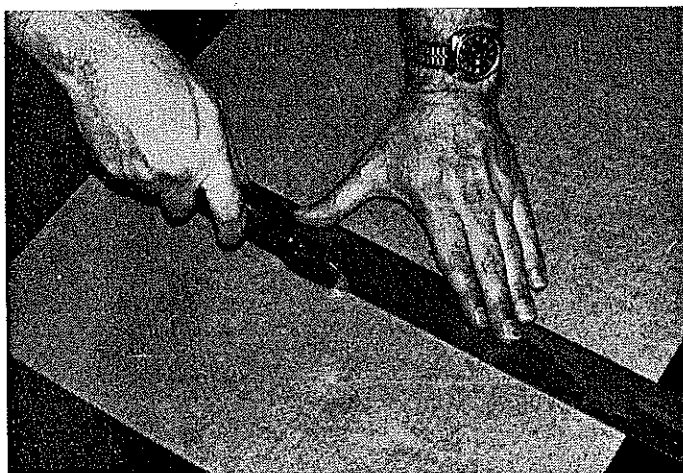
This is how to score corrugated cardboard for making folds. It takes a screening tool and metal straightedge.
