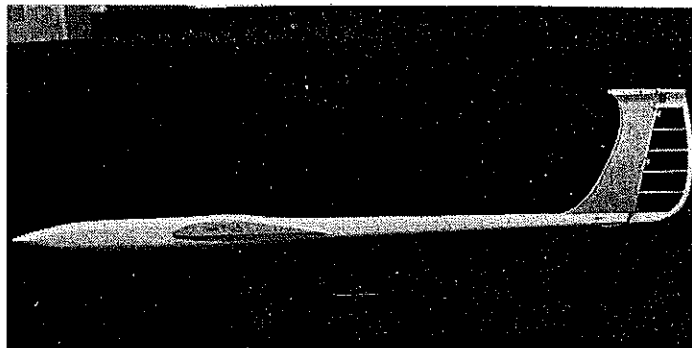
Fuselage ready for covering. An iron-on film, such as MonoKote, is recommended for saving time and weight vs. paint. To comply with current AMA and FAI rules, model's nose must be rounded to 7.5mm radius.
