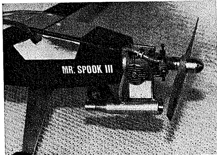
Both .25 and .40 engine installations are shown in these pictures. Interchangeable round radial mounts were used. Match the mounting holes of both mounts so that a single set of firewall blind nuts can be used. Screw in front of wing holds tank access hatch in place.
