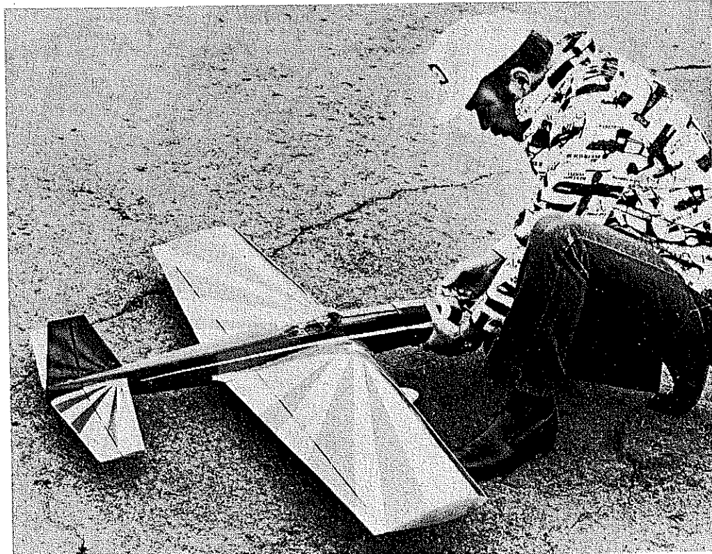
In spite of the way the author's dressed, the temperature was 25 deg. Things start reluctantly in that weather. Super Star's inverted engine mount allows easy engine access.
