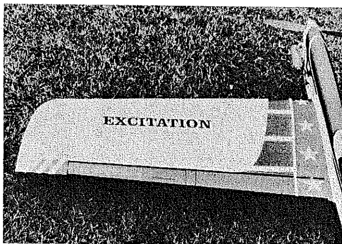
Slightly tapered flap is a constant 17% of wing chord. Lines and details were done with a Rapidograph technical pen, available at art stores.
