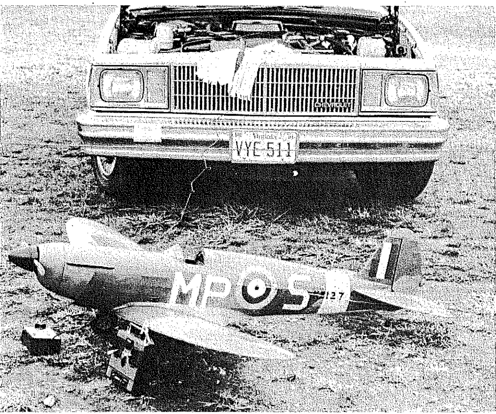
The Spitfire fuels up between flights. Connect the charger to the plane and to your car battery, set the timer to 15 minutes, and walk away. Full charge gives about eight minutes' flying.
