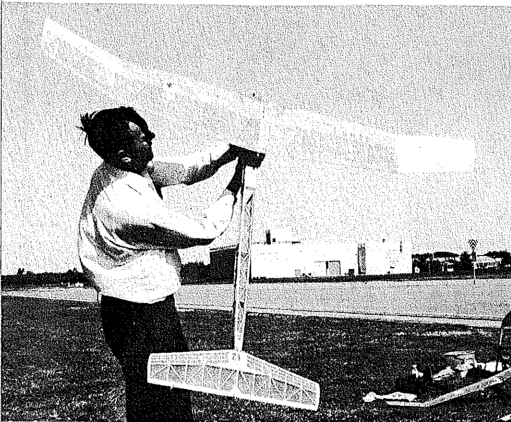
Author peaks out the engine prior to launch. Note that tweaking is being done in climbing attitude. For maximum rigidity, wing is covered with silkspan, then with 1/2-mil Mylar.
