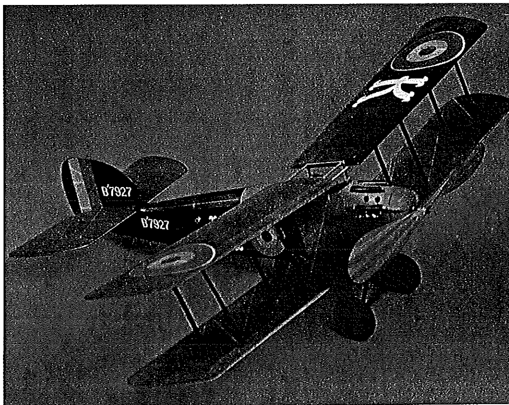
Author recommends Peck-Polymers prop—8-in. dia. If takeoffs are planned, 9-in. for better performance if hand-launching. Uses four or six strands of 3/16-in. rubber for power.
