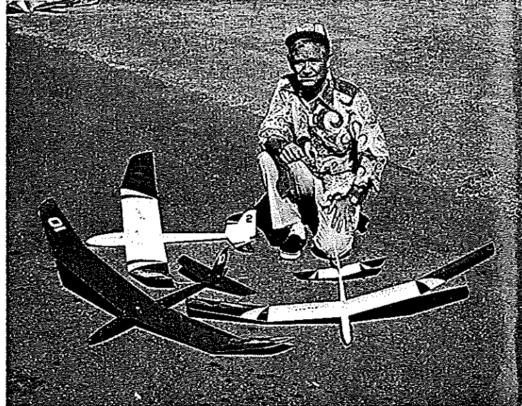
Three different versions of the Zephyr in this view. Headed straight at us is the first one, with a conventional tapered wing. Number 2 is the subject of this article. Red job is the heavyweight at 13 oz.
