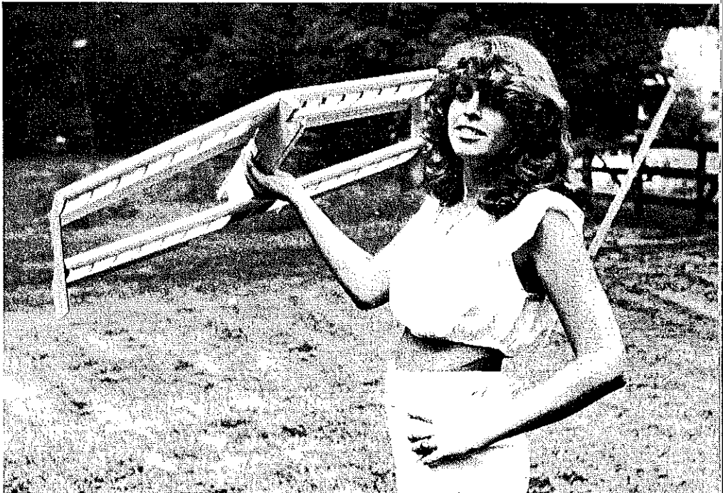
The author's daughter, Mary Carol Hunton, holds the framework of an earlier version which had a tandem wing and tandem engine. Twin engines abandoned due to trouble of starting both engines.
