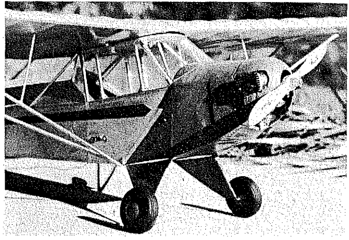
Unique cabin structure of the E-2 shows in these pictures. Optional side window panels were available to keep the cold wind out in the winter. In photo at right, note how plenty of cooling air and easy access to the engine are provided by the cut-out in the bottom of the cowling.
