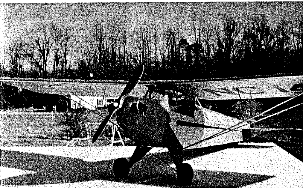
Removable cowl with dummy Continental 40 engine camouflages the inverted Cox .049 engine. Minimum dihedral helps scale appearance, and provides adequate stability for rudder-elevator controls.
