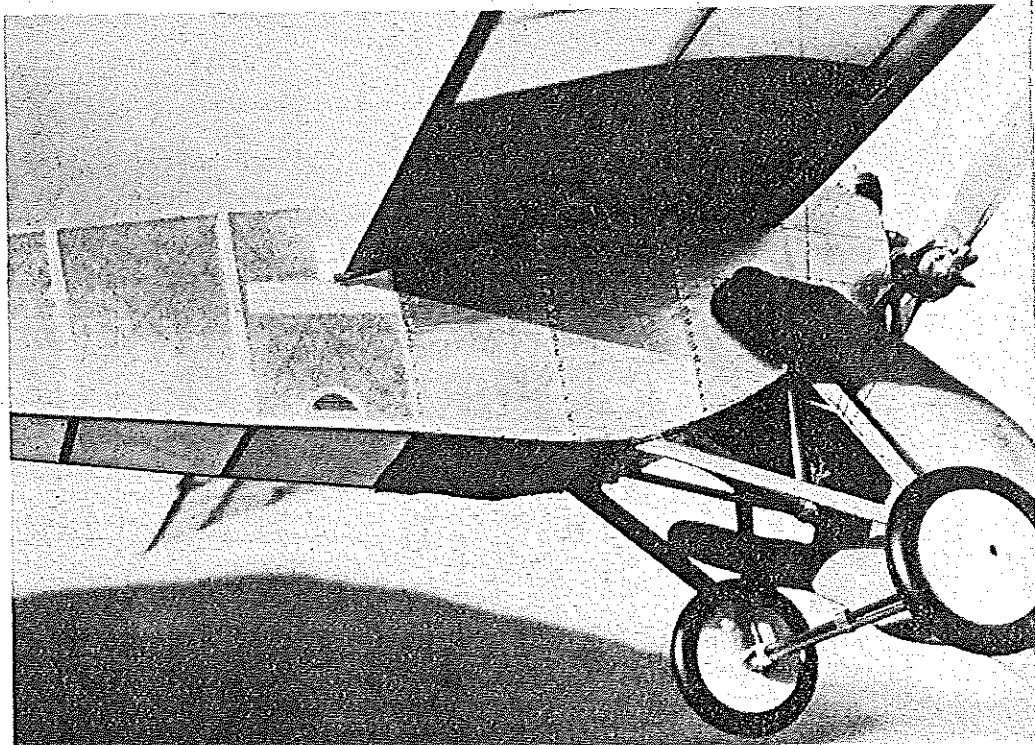
Detailing seen from below includes the step, aluminum panels, and black thread cross-wires in the fuselage—fair amount of work, but looks oh so good when the model is circling lazily overhead.
