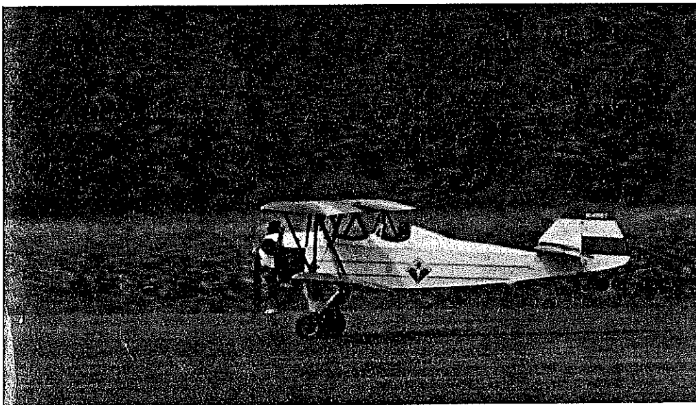
What we all love to see—a classic biplane, tall just up, rolling faster and faster on really smooth grass. With 840 sq. in. of wing area, the wing loading is a pollite 13.4 oz./sq./ft.
