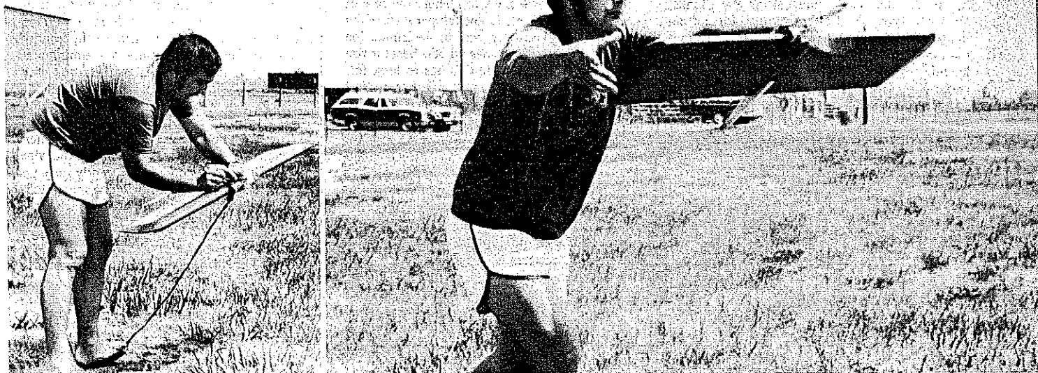
And now that the engine is running, the author maintains the same one-handed grip, left, as he tweaks the needle for a just-so mixture. At the right, he demonstrates the traditional launch. Note the angle of the ship and how both hands have just been lifted free.
