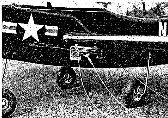
Bellcrank detail: Roberts Suspended 3-line bellcrank fastens to homebrew metal mount which then attaches by bolts going through fuselage.
