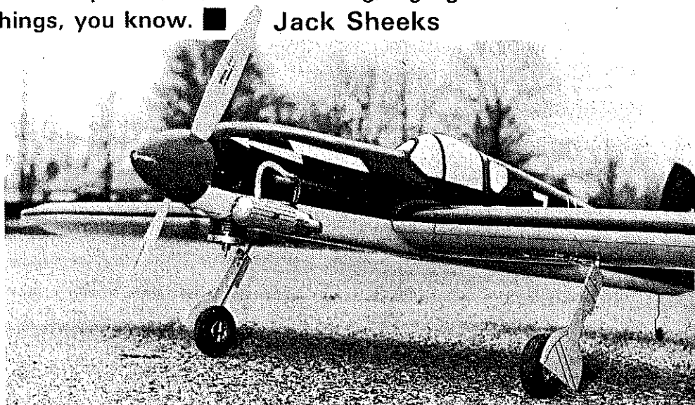
Pugnacious and clean, Jack rates his 100 a fine-flying stunt ship—and goodness knows, he is the most prolific of designer/builders. Plans show Max 35—ship takes 35 to 40 power, and Jack used an HB 40. If you elect the HB, slight mods are required in the nose, but are explained in text.
