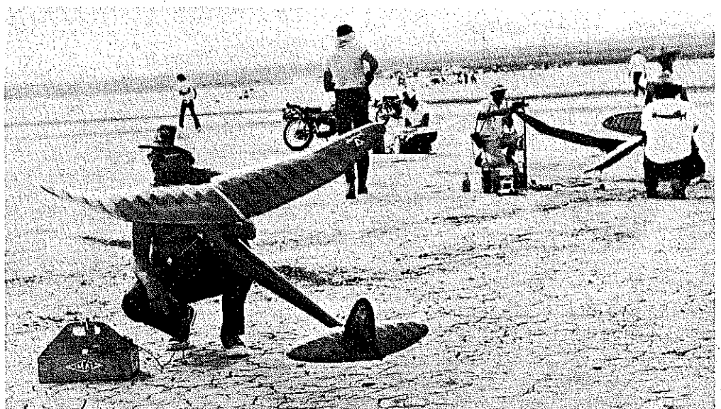
Uncommon Super Viking, designed by Don Wencell, has sweeping graceful lines. Note relatively small stab and recessed leading edge at the center of the wing. This version, by Mitch Post, is powered by a Super Cyclone engine. It has an impressive idle.
