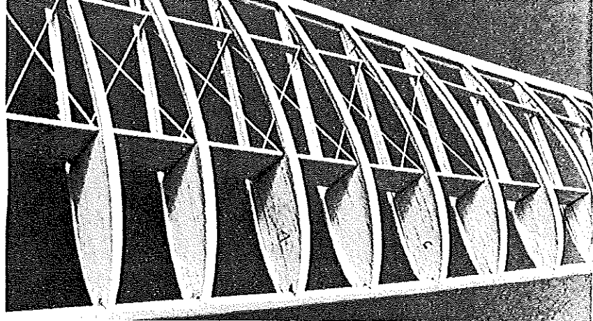
Left: Wing panels are slipped in place, with the stub spar extending to ply spar joiner in the center section. Right: Rib and spar details suggest that the wing frame has a high strength-to-weight ratio. Cap strips yield better appearance but may be left off if maximum duration is your game.
