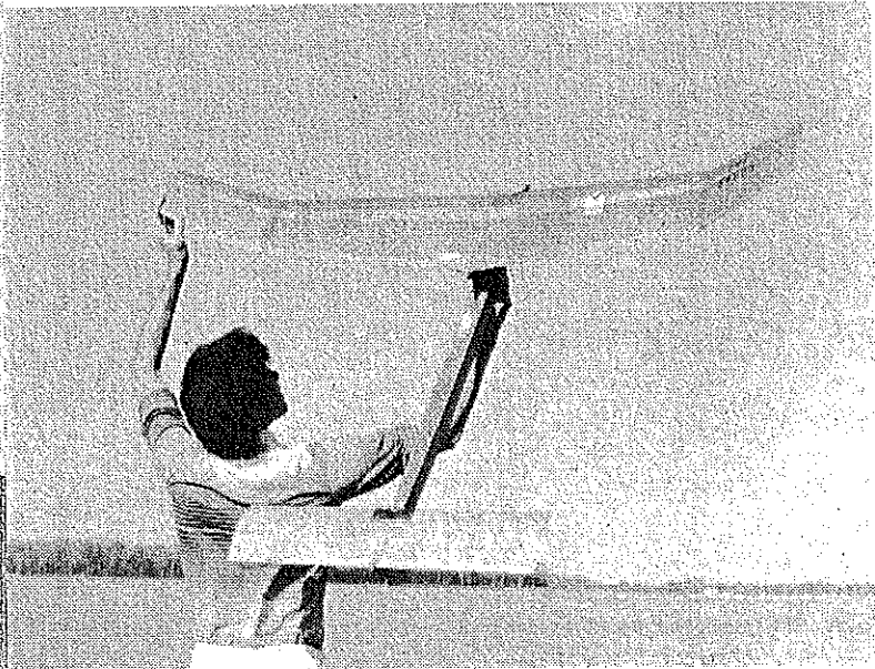
Original Class C experimental job from which Toothpicks was derived. Souped-up Fox 36 single by-pass, and 580 sq. in. wing. The design stressed concentrating real weight elements as close as possible to CG—involving very light tail, and engine pulled back. Refining that approach had evident beneficial effects on both the transition and glide.
