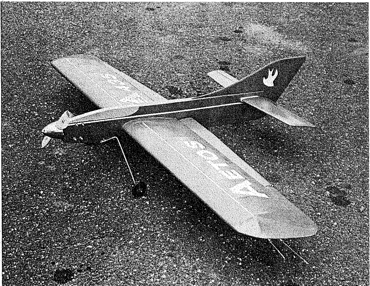
From the left side, other details are visible—landing gear attachment, lead-out guides, showing bit of up flap coupled with down elevator. Especially note indication of thickness to profile fuselage. Roger uses simple "hollow" construction—looks better and is quite light.
