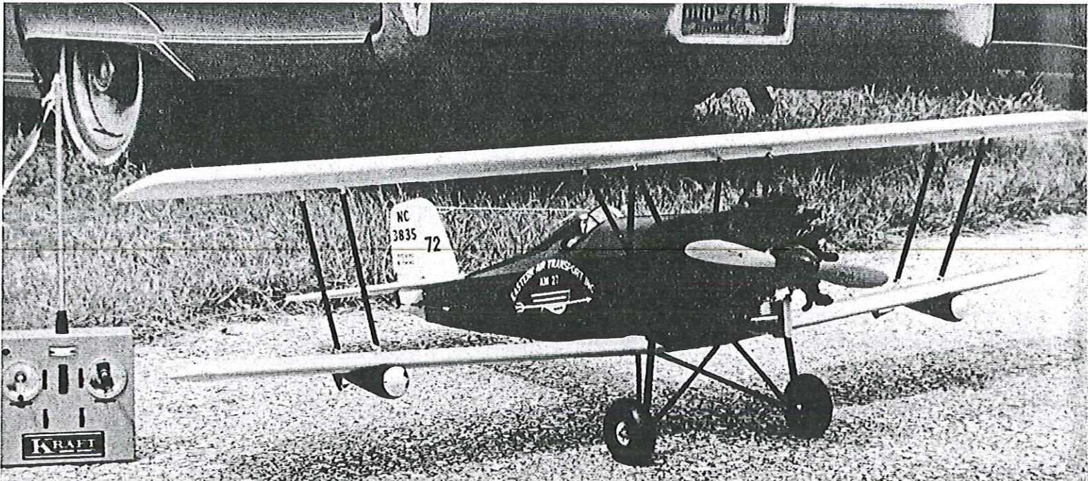
With its flying propeller installed, the Mailwing awaits its first test hop. The builder is urged to observe the offset and downthrust angles of the motor mounting (see Fig. 1). Wings are covered with yellow Coverite, fuselage in black. The 12-oz. sq. Sullivan tank fits within a quart-size milk container which is positioned to hold the tank.
