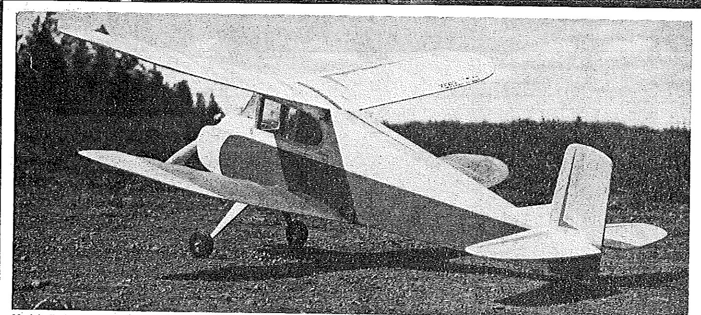
Model climbs at angle shown at instant of launch, in left-hand turns. Turn adjusted by increasing or decreasing built-in left thrust, climb by more or less down thrust. Insert: Reminiscent of Waco biplanes of the Thirties, Dakota's generous wing area allows heavier construction. Dihedral provides good stability. Though purposely heavy to avoid fly-aways, the Dakota should not be flown in areas of known strong thermal activity.
