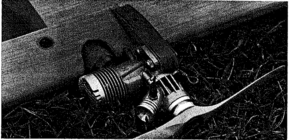
Closeup of Doss Porter's plane showing engine/exhaust layout. Note safety cable that will be hooked to engine to keep it from coming free of the plane in case of a mid-air or a mount failure. Other end of the safety cable is attached to the bellcrank. Photo by the author.
